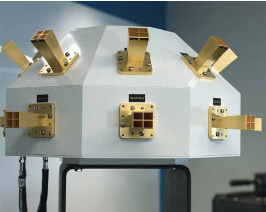
AT&T developed the “Porcupine” antenna with NI to do real-time, detailed 5G channel sounding.
