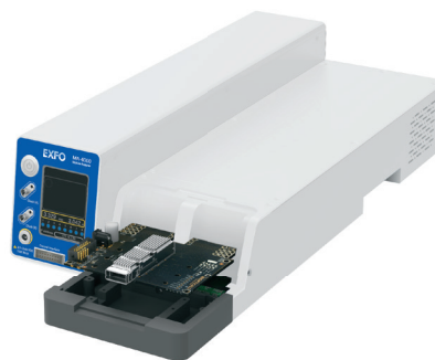
Easy-to-replace MCB in direct contact with BERT
